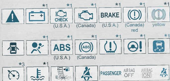
\*1: These lights turn on when the "POWER" switch is turned to ON mode to indicate that a system check is being performed. They will turn off after the hybrid system is started, or after a few seconds. There may be a malfunction in a system if the lights do not come on, or if the lights do not turn off. Have the vehicle inspected by your Toyota dealer.
