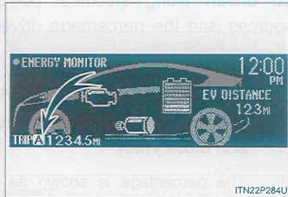
The display changes as follows each time the “TRIP” button is pressed.
