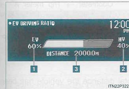
**1** Percentage driven in EV mode using the electric motor (traction motor) only
