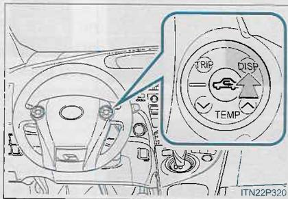
Press and hold the “DISP” switch while either the 5-minute interval or 1-minute interval display is being shown.
