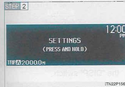
While the vehicle is stopped, press and hold the “DISP” switch until the screen changes.
