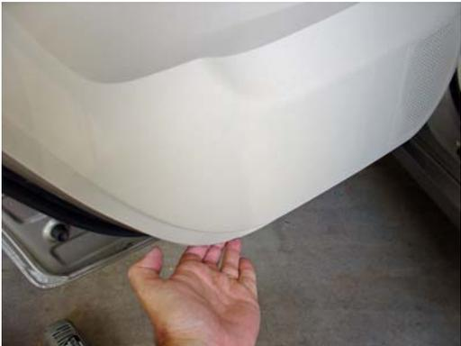
Continue unsnapping panel around the bottom and up the sides; when fully unsnapped, lift panel up – be careful to not scratch windows (especially if you have tint).
