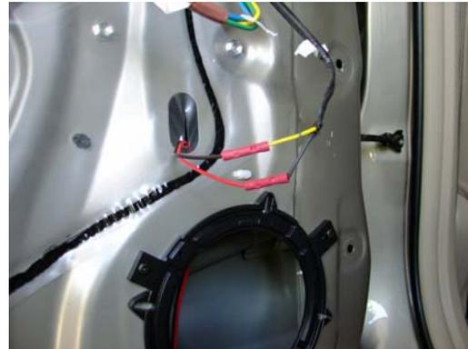
Connect wires (make sure to confirm +/- polarity) – my connections as shown were to a crossover. The car's black is + and yellow is -, connected to my crossover's red + and black – (always interesting not connecting black to black...)
