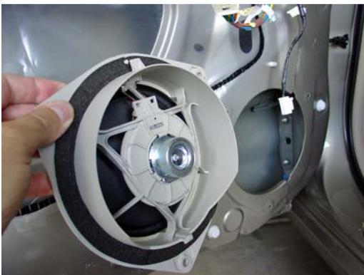
Remove the speaker – amazing how small the magnet is on the back is, and how light the entire speakers is – *no wonder it sounded like that !*
