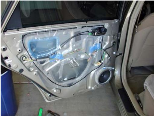
Photo of door with panel removed. I had a few *stubborn* white clips stay in the door – remove them from the door by pushing from the inside out – and re-attach them to the door panel.
