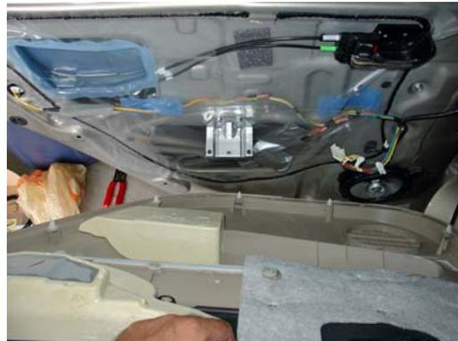
Attach the door panel to the door – press gently at the points where the white clips fit back into the door. They should snap easily into place.
