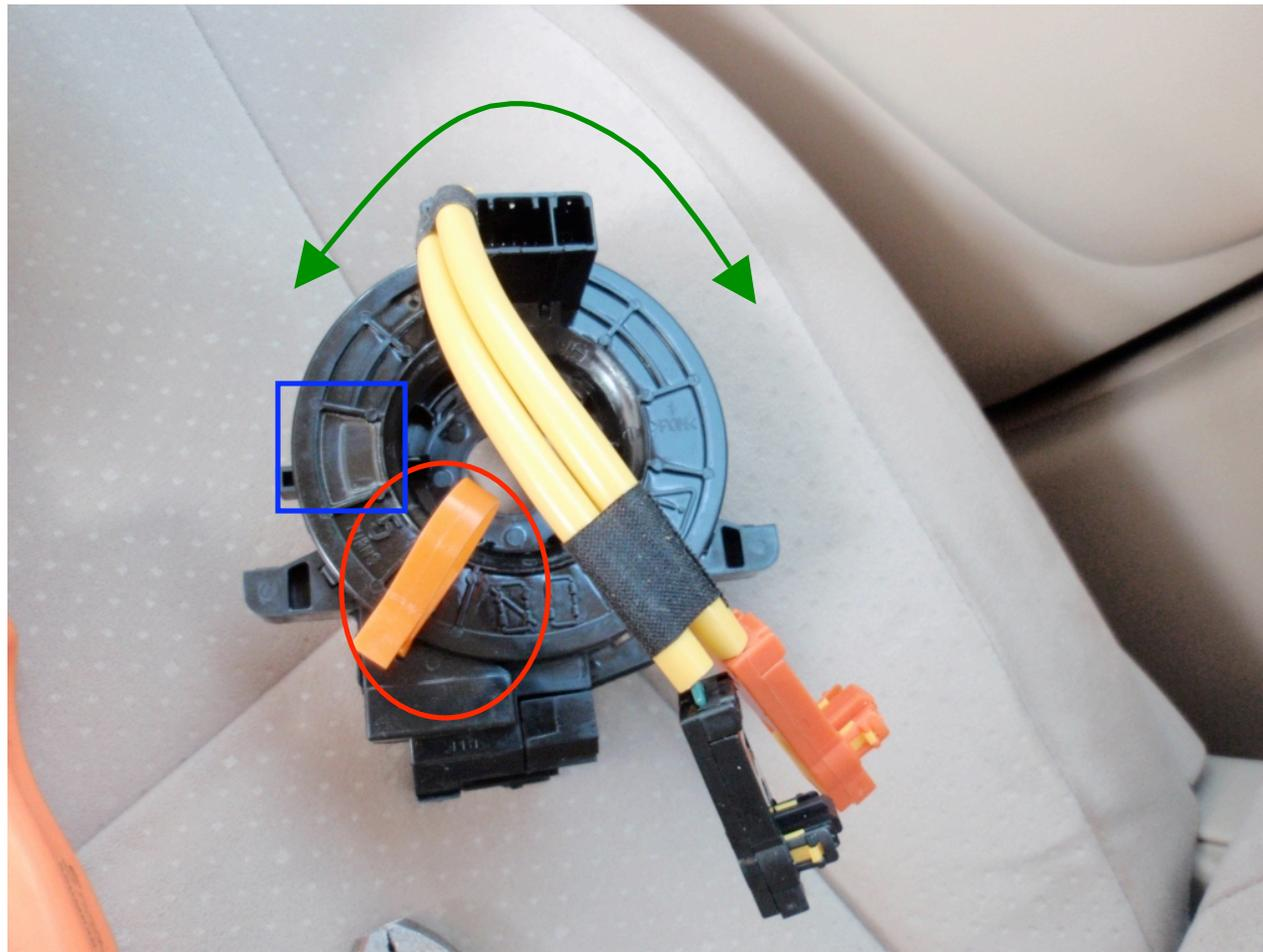
Make sure you either **transplant the steering sensor** from the back of the old clock spring assembly or make sure your used replacement has it already installed. It is held on with more small plastic “latches”. It indexes with the front half of the clock spring to tell the Prius which way and how fast you're turning the wheel. **Make SURE you have this installed before re-installing the replacement clock spring!**
