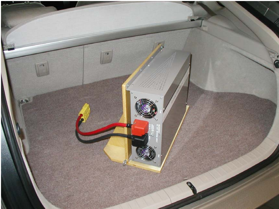
The Inverter is mounted to a plywood support frame
