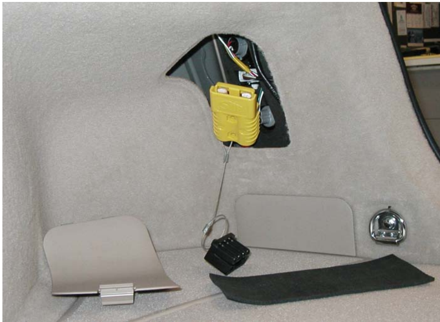
The Anderson connector is just behind the right-rear access cover. Note the black “dust cover” for the end of the Anderson connector (on a retention cable). Also, a rectangle of foam rubber is wrapped around the Anderson connector to minimize any rattling noises
