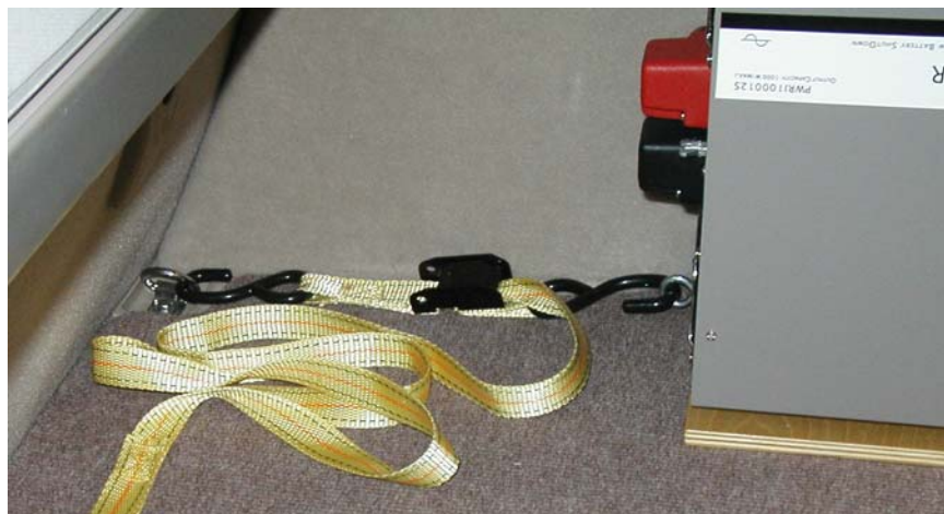
A tie-down strap between another Prius D-Ring and a screw-eye in the plywood, also secure the inverter in place
