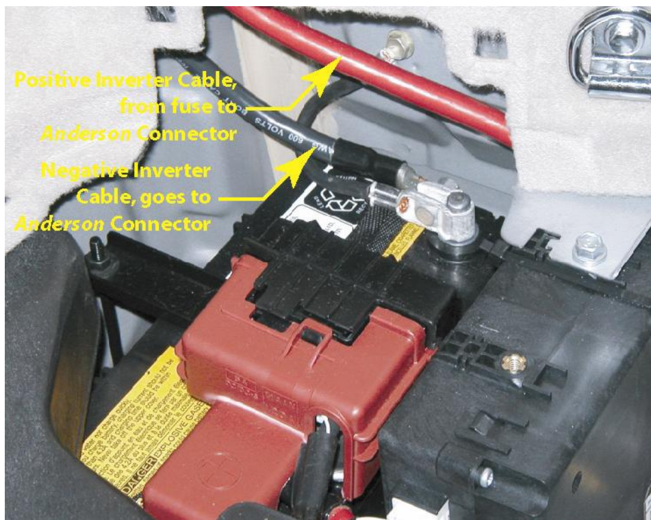
A view of the Prius 12 Volt battery, with the Negative cable attached
