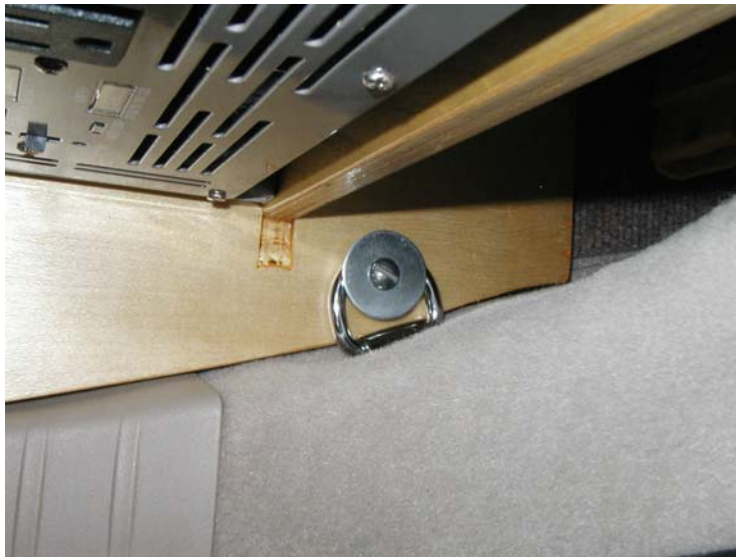
The plywood has threaded insert. A bolt with large washer, screwed through the Prius D-ring holds the inverter in place
