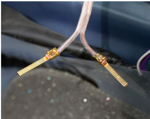
Figure 12: Left: Flat pin connectors to insert into factory wire header receptacle. Right: Pins inserted into passenger side receptacle.
