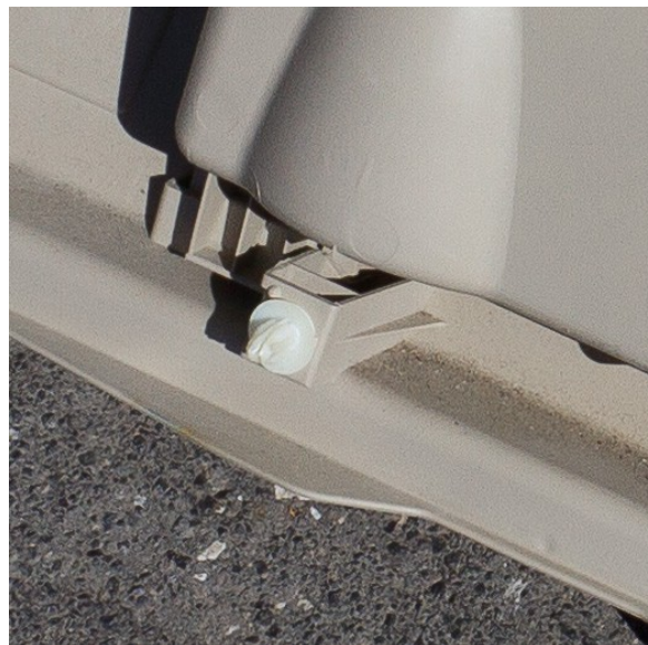
Figure 5: White retaining clip still in door panel as it should be
