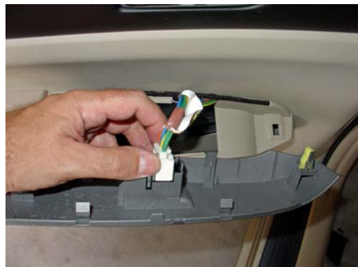
Disconnect automatic window switch.
