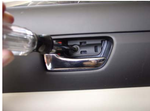
Remove small plastic cover panel and screw #2 in door pull.
