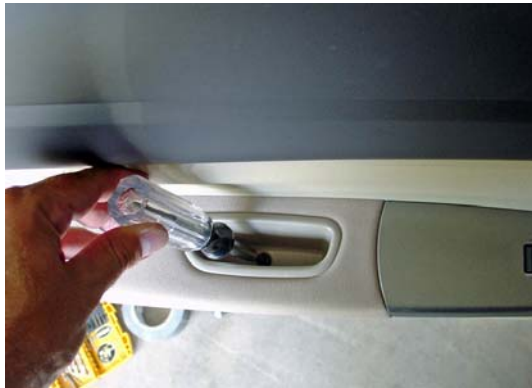
Remove screw #1 in arm rest panel.
