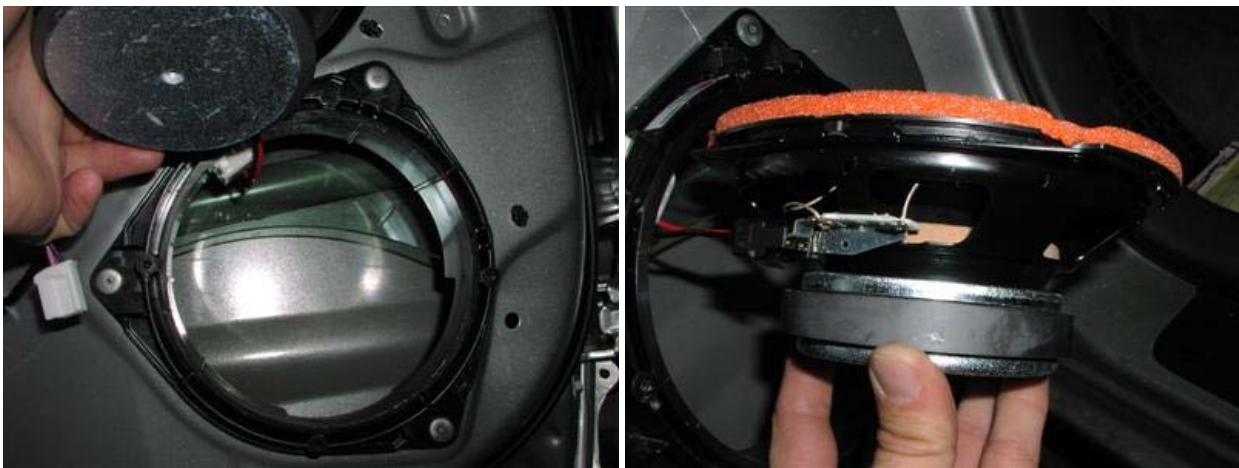
Front door woofer off. Window rolled all the way down. Notice glass 3" away from mounting lip would prevent very large magnet speakers from being used.
