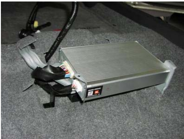
Left: The JBL Amp, as seen with the black plastic cover removed and the passenger seat removed. Right: JBL amp removed, exposing
