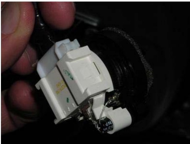
Left: the back of the tweeter assembly. Notice the black capacitor on the rear tweeter. Right: Right Rear tweeter connector
