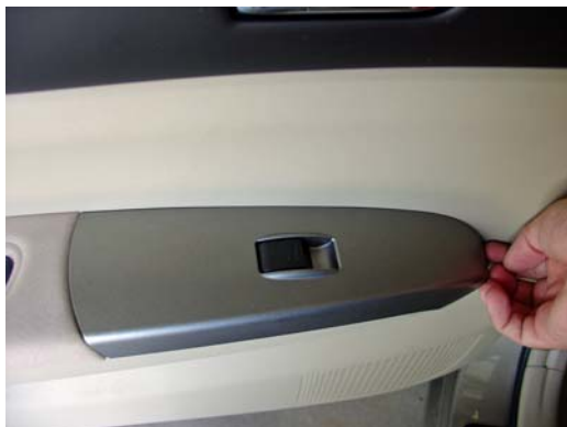
Remove arm rest panel – up gently on forward edge – it snaps out very easily,
