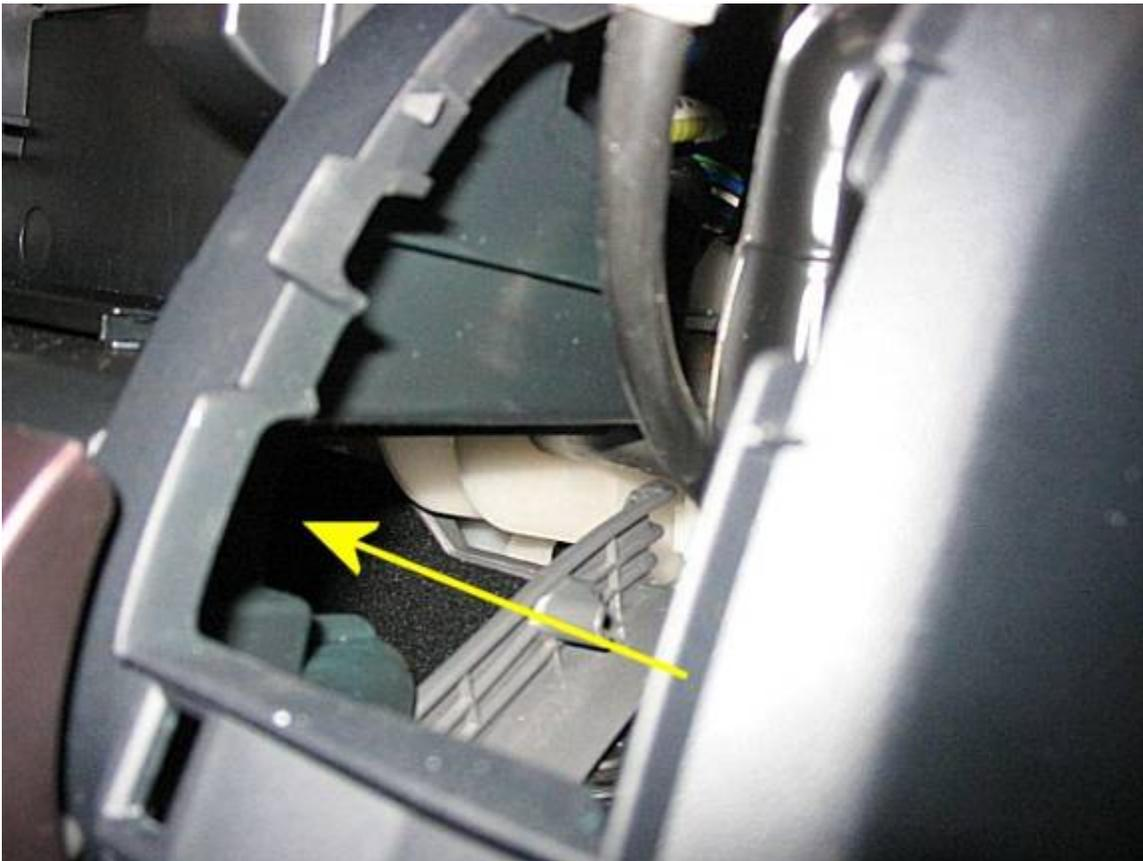
**Open and lower the glove box, to make sure of cable placement.**
