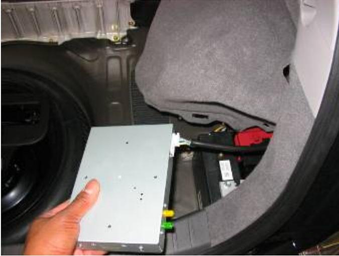
**Make sure your plugs are facing down and not up when mounting. Find the flattest surface possible. There is a prime spot just above and ahead of the battery.**
