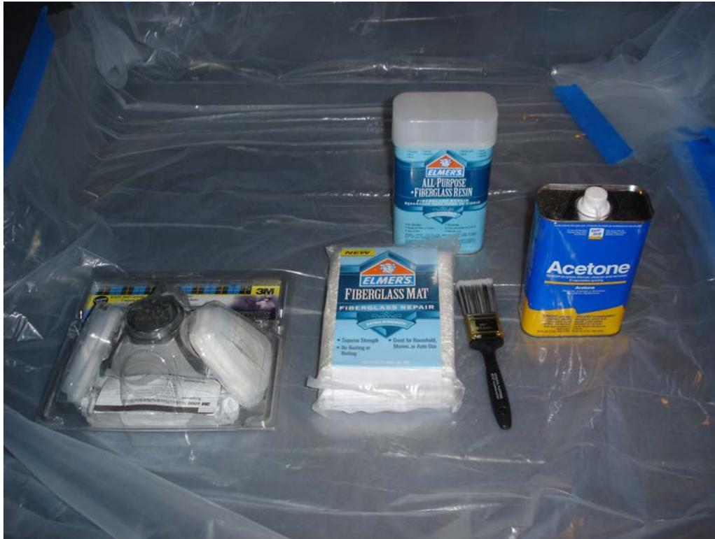
Pictured here are a respirator mask, fiberglass matt, fiberglass resin/sealant, paint brush, and acetone for cleaning the brush. Additionally, I purchased grey car fabric from [www.partsexpress.com](http://www.partsexpress.com).
