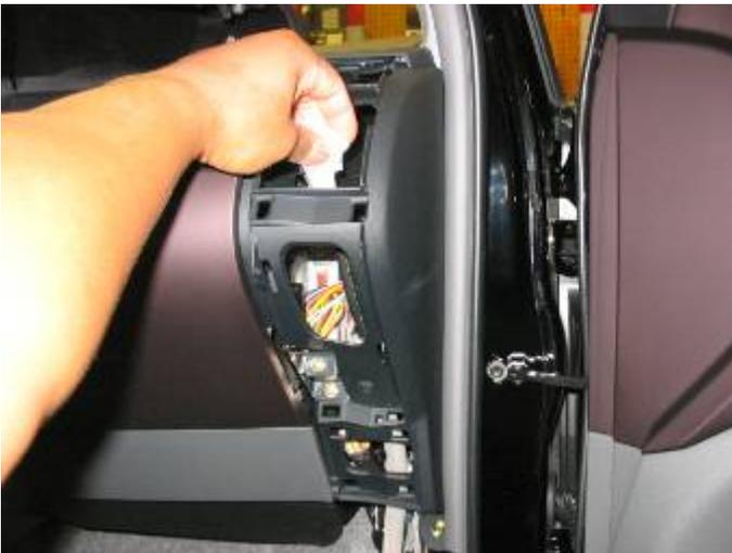
**Feed the cable out of the register hole. You really only need to pull enough cable to make it to the radio assembly.**
