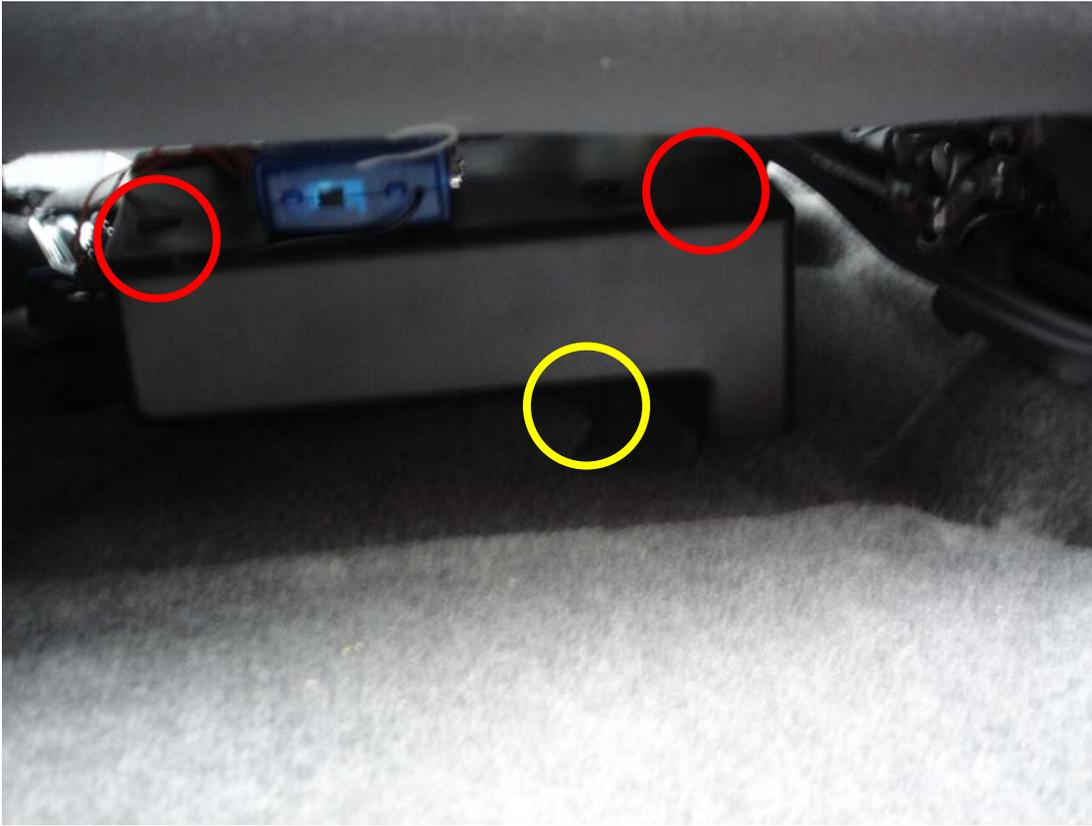
Above, the red circles indicate the location of the two plastic bolts, and the yellow indicates the location of a rear bolt that holds the amp to the floor. This bolt is hidden beneath a piece of carpet that easily pulls back.
