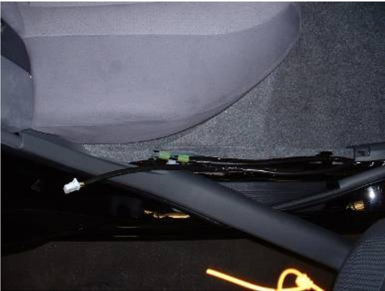
Here you will see that the rear seat is removed. It is not absolutely necessary but it is so easy to do and makes the install a little easier. The front of the rear seat pops into these plastic clips.
