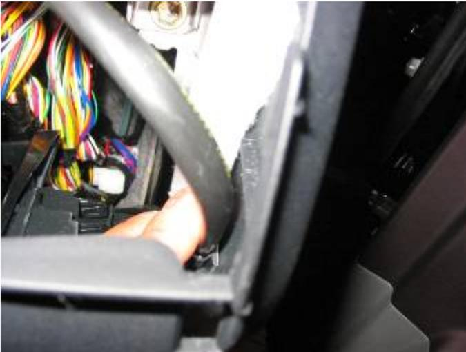
**Be sure the cable is pulled taut. What we are trying to do is have the cable not interfere with the glove box door. Be sure to check it's operation and make adjustments to the cable as needed.**
