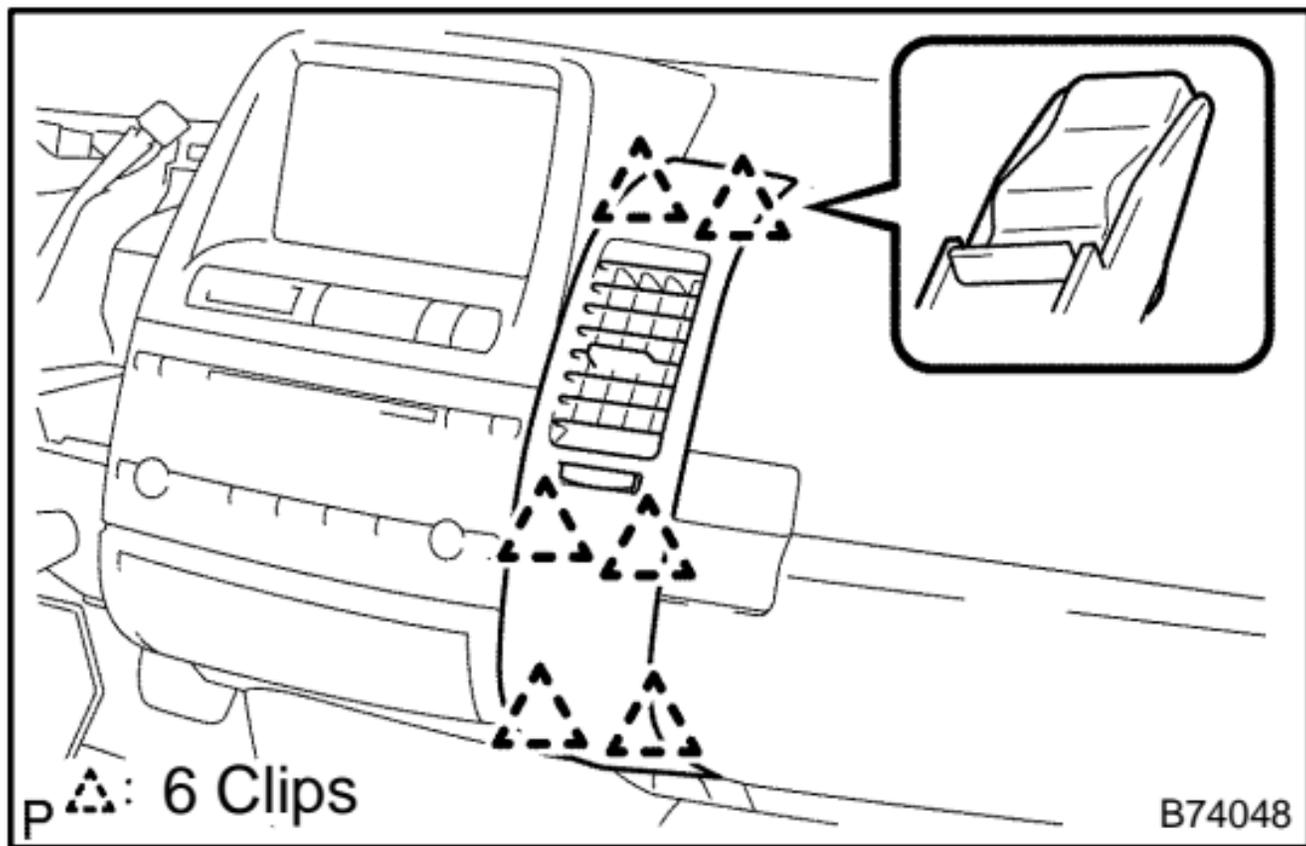
**REMOVE INSTRUMENT PANEL REGISTER ASSY
