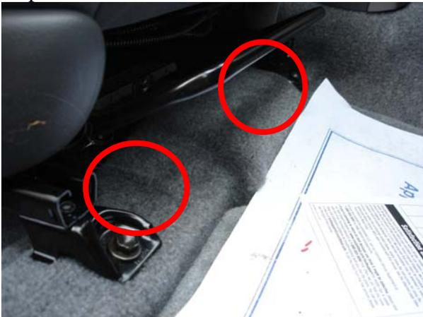
Note: The two bolts you need to remove from the front are beneath two flaps of carpet just inside of the bolts holding the seat to the car.
