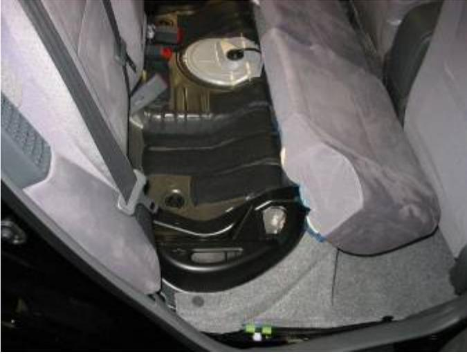
**Fold down right rear seat. Remove cargo cover, spare tire cover and cargo tray. Peel back carpet (velcroed to seat back).**
