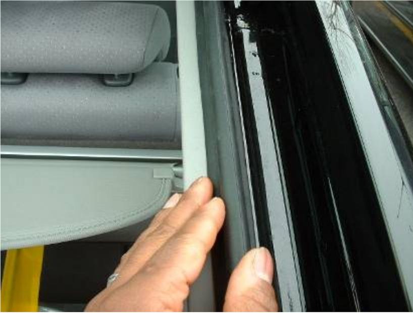
**Refit all of your panels. Replace the carpeting, cargo and spare tire covers. Replace the sill plates and any other items removed.**
