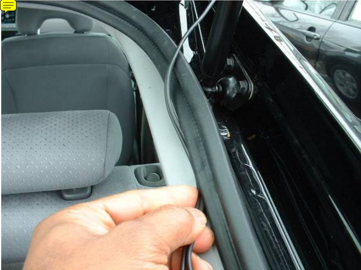
**Route the antenna wire behind the right finish panel. Plug the antenna into the XM radio unit. Test the XM radio operation once again.**
