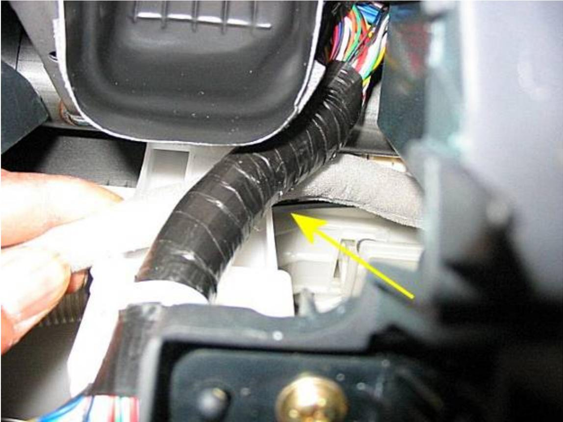
**Make sure to run the XM radio cable under this bundle of wires.**
