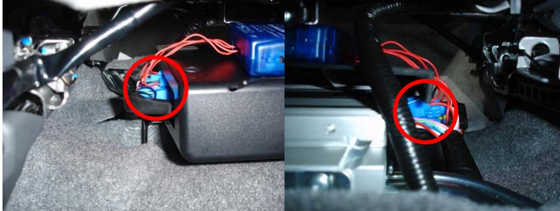
Note: The light blue plastic fittings above are the line taps. They fit over the current wires and simply require crimping to work. You don't have to cut any wires!
