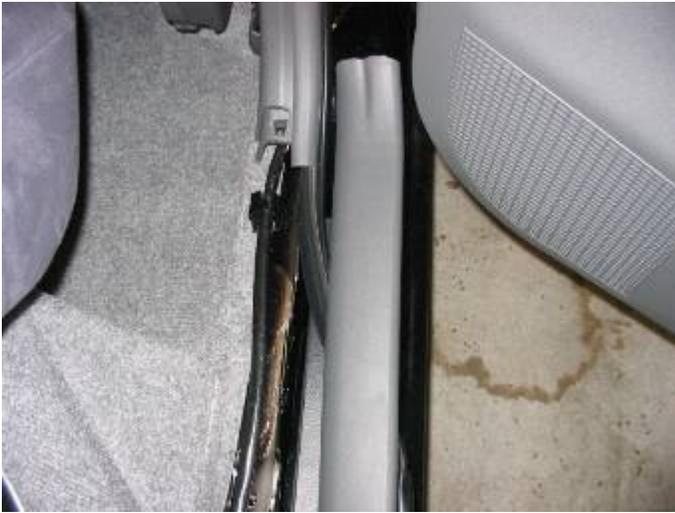
**Pull the weatherstrip away from both sides of the B pillar panel (You know, that plastic panel between the front and rear doors).**
