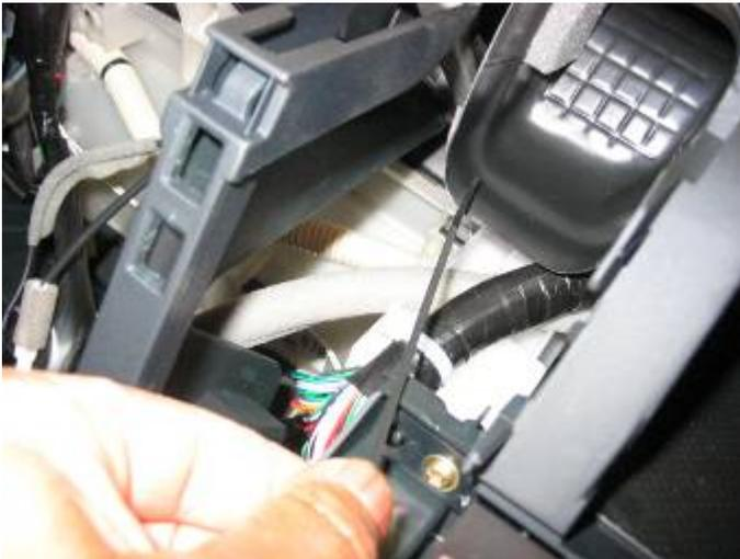
**Leave enough cable to plug into the radio then tie the XM cable off with one of the zip ties located in the XM radio kit.**
