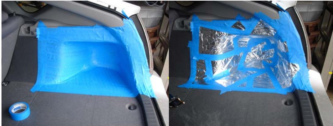
In addition to prepping the immediate area, you should cover the surrounding area with a thick plastic dropcloth. The plastic will ensure that any spills or splatters will not get on the carpet.
