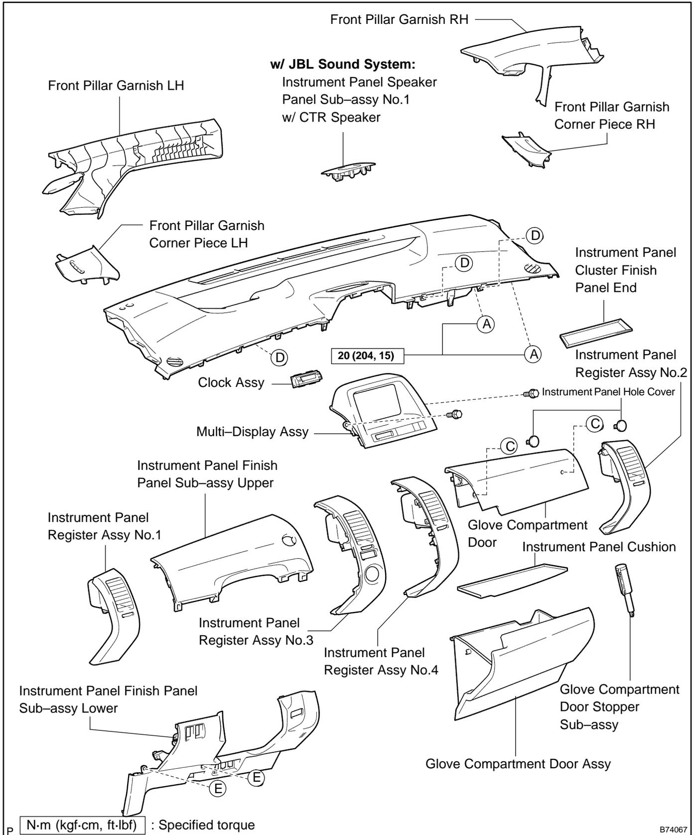
**REMOVE INSTRUMENT PANEL REGISTER ASSY
