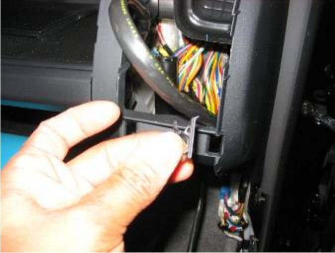
**There is a special cable tie in the kit. It has sticky tape attached to it. Put the XM cable into the tie then stick the tie to the inside of the dash by register No.4.**
