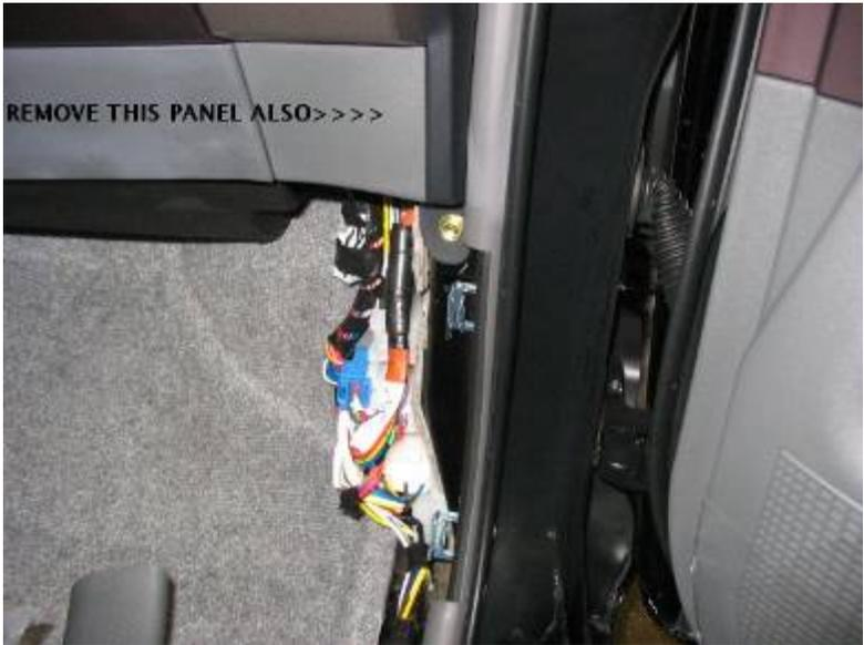
**Take the cable from the XM radio kit foam side first and feed it behind the dash.**
