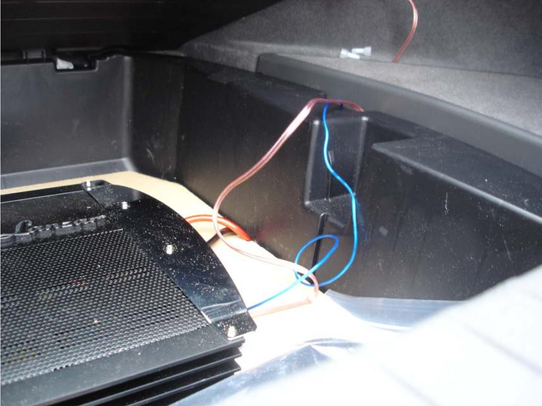
Note, here you can see the power wires, remote wire, and speaker wire.
