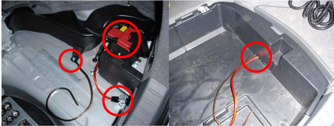
The circles above indicate the mounting pointed for the positive and negative ends, as well as the plastic fuse holder and the holes drilled in the plastic tray to allow the wires in.
