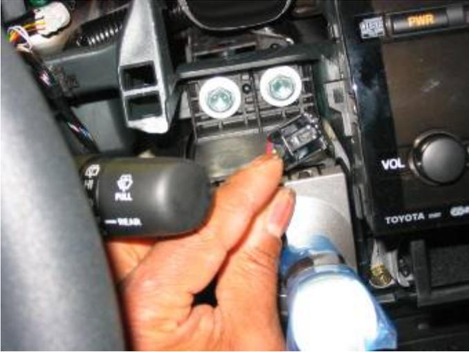
**REMOVE INSTRUMENT PANEL REGISTER ASSY
