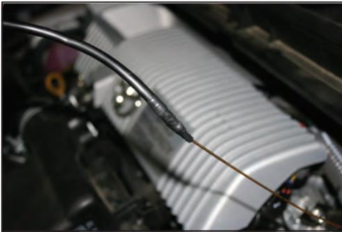
**STEP 6.5** **IMPORTANT!** Wrap electrical tape around connector, tubing and rod. It is important that all three be secured as one unit so not to rip connector from wiring. You want tubing to take as much of the pull force as possible.
