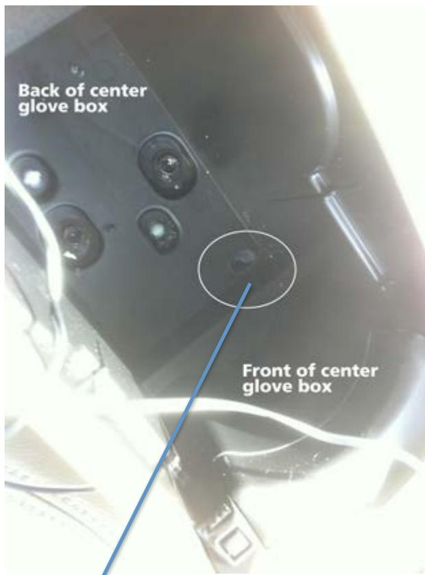
Drill a small hole in the bottom of the center glove box and run the power and aux wires along the console and into the lower glove box. **Feed wire through to center column through here.**
