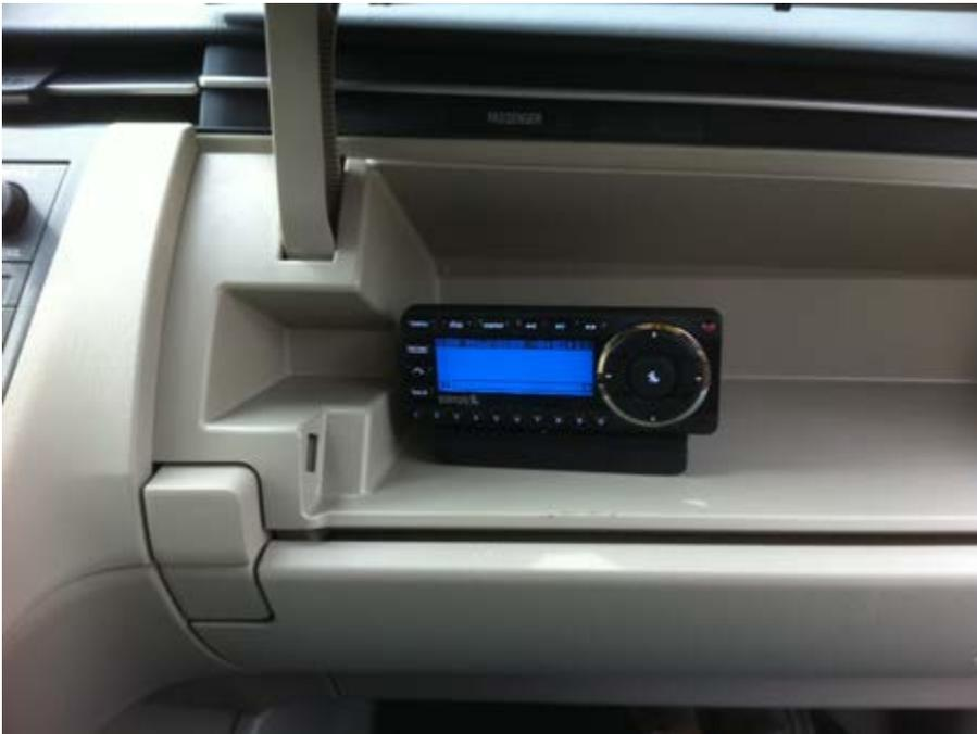
I mounted my unit with bolts through the bottom of the upper glove box, This is easy because the entire glove box comes out.
