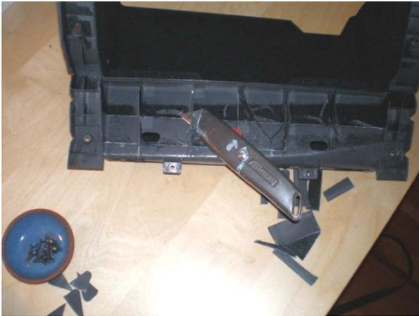
After separating the two pieces, I started working on the bottom half by removing the fins that hold that shelf in place.
