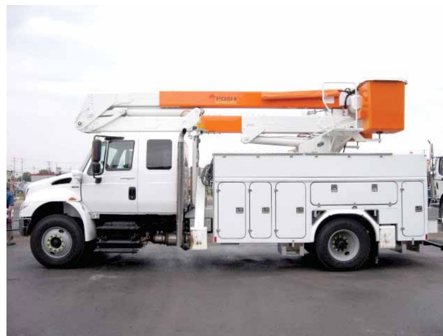
A truck equipped with an electric-hydraulic man lift developed by Posi-Plus
