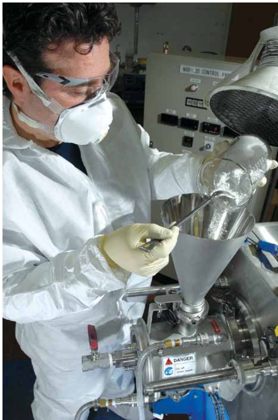
Work underway at IREQ on eutectic salts for lithium-ion battery production
