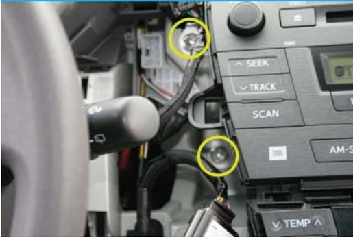
Step 2. Remove the mounting bolts on the passenger side.
