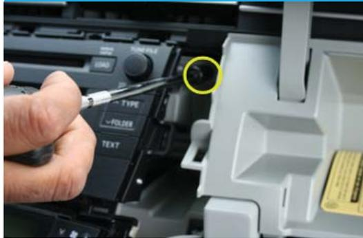
Step 3. Remove the mounting brackets from the factory radio.
