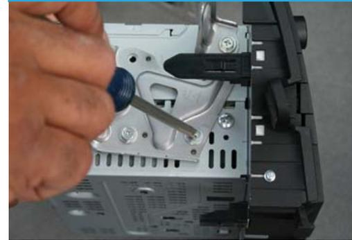
Step 4. Install the mounting brackets on the M&D radio.
