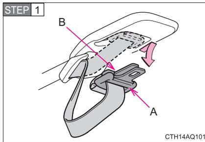
Push the tabs back all the way into the cover and then remove the tabs.
