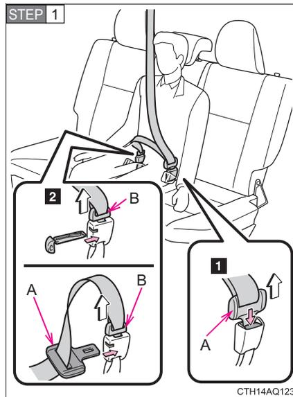
**1** To release tab “A”, press the release button.
