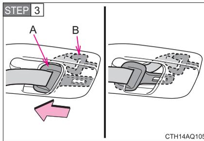
With tab “B” inserted all the way into the cover, move tab “A” slightly back toward the cover’s inlet, so that it blocks the inlet.
