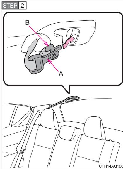
Holding tab “A” and “B” together, insert both tabs all the way into the cover on the roof.
