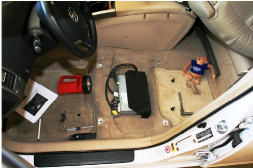
under the seat, it's always good to get adequate lighting, especially for us far sighted folks. The yellow arrows pictured point to where the NEW mount holes are ... 4" back from the hex heads where the original mount holes are. The original metric bolts get put back in loose, for wiggle-room. Similarly, when you drop the seat back into position, the 4 new 3/8 bolts get put in loose.
