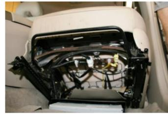
Newb's should read for example, "On the far left connector, push the blue dot in ... push in the square button on the center module ... slide the white slider on the yellow connector; slide it towards the black wire jacket" ... or something
