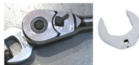
I used a 'crowsfoot' wrench. This has a claw feature of an open end wrench, but offsets to ratchet or torque in hard to get at places. Stick your ratchet
