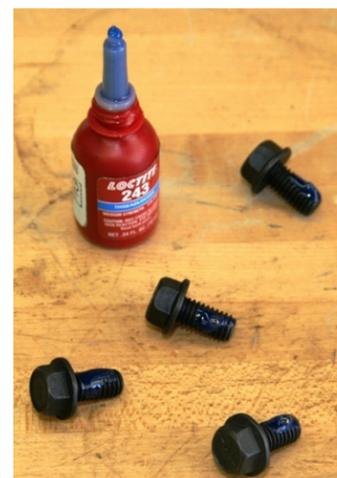
Now, in comes Loctite (see dabs of dark blue on the bolt threads pictured above). Before it hardens, it acts as a lube. Wet threads give higher clamp load even at lower torque. This means you can use over 20 lbs less torque during installation! Less torque is a GOOD thing if you have limited thread penetration. FYI, Torque is how tight your bolts are.
