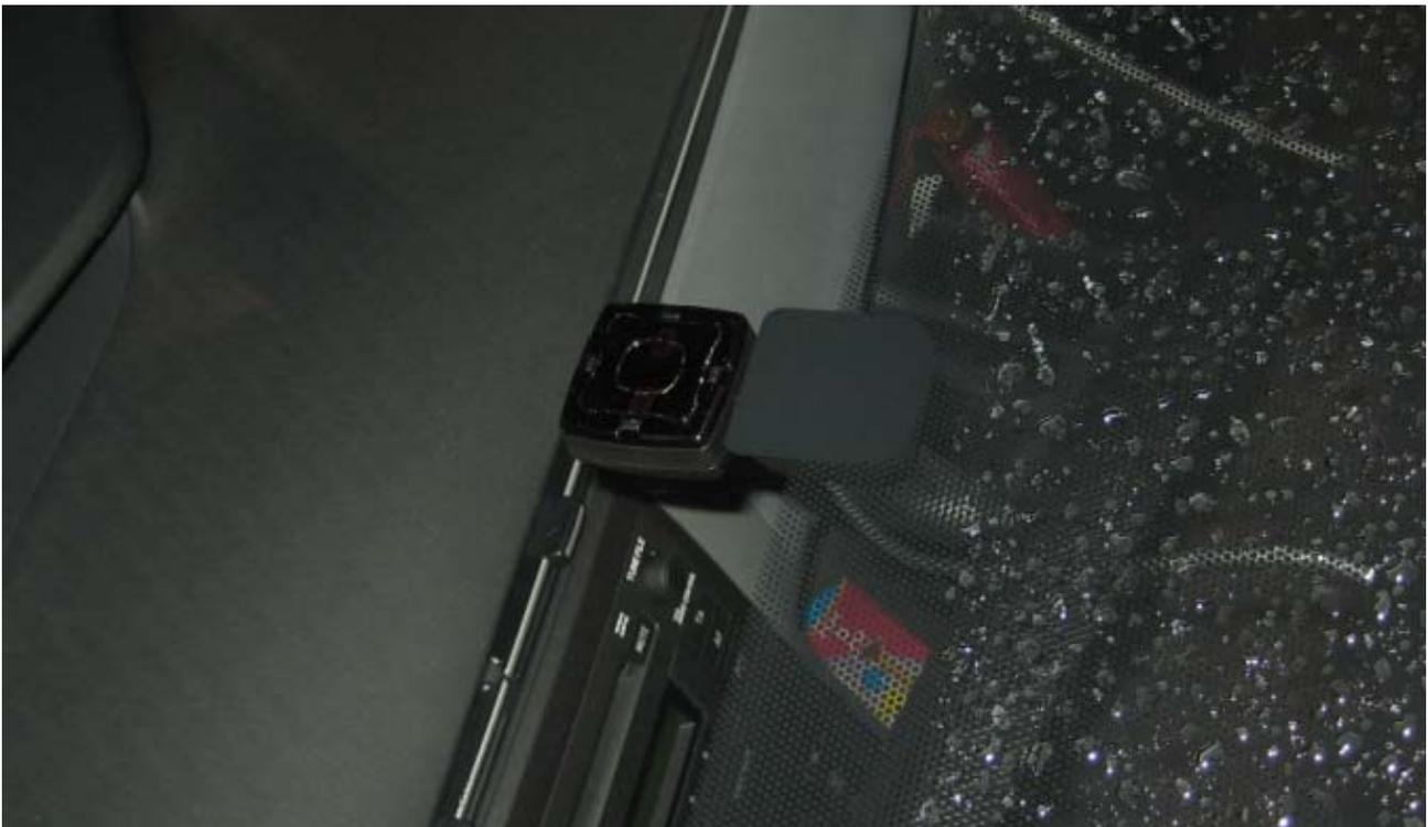
When calculating the space between sensor and mirror, consider also the length of the sensor socket. In the following picture, the sensor socket had to be twisted due to lack of space. It would be better to avoid this operation, even if not influencing at all the electric connections and not compromising so much its mechanical performance.
