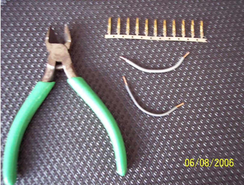
Figure 6. Strip insulation at ends of wires.
