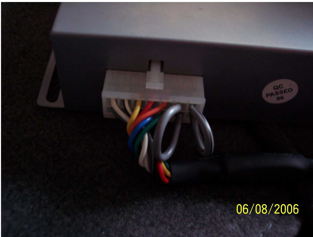
Figure 10. Properly installed jumpers.
