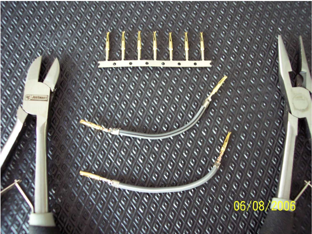
Figure 8. Use needle nose to crimp connectors on to ends of wires.
