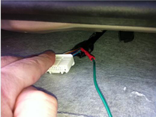
Once the wire is connected then guide the wires back into the connectors in the roof and clip them back in, then route your new wire over to the passenger side above the headliner. I pulled off the top part of this trim piece...
