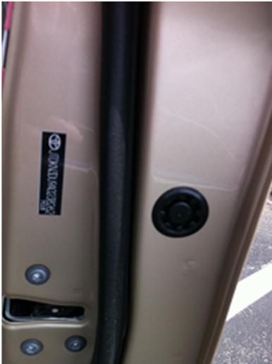
Remove the plug to expose the screw behind it.
