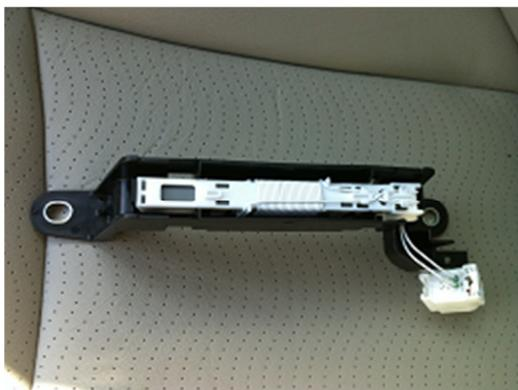
Cut off the connector and use the butt connectors to attach wires to the antenna. Since the antenna gets mounted outside the car I would suggest using weatherproof connectors. The ones I used came with heat shrink tubing over the connector, so after crimping it down I used a lighter to shrink the tubing... the lighter burned it a bit, so you can see some soot on the connector. Oops.
