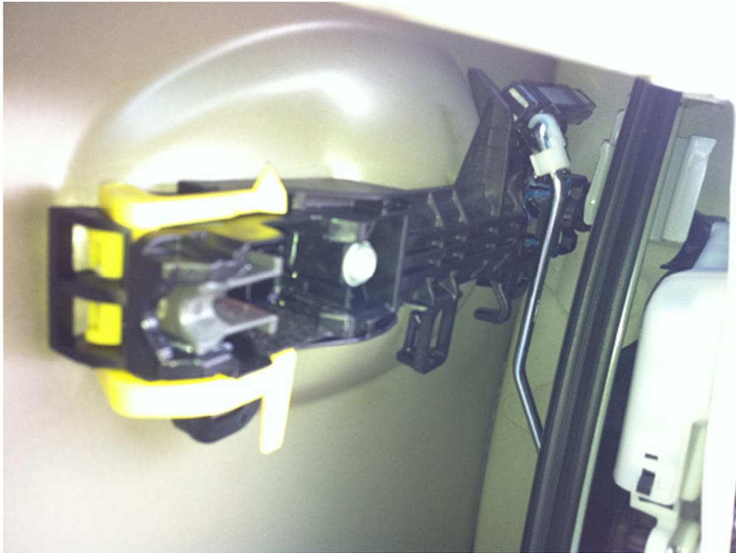
Below is a picture of the wiring harness installed correctly. Note that there are two white plastic locks that get pushed into holes in the black handle to hold the harness in place. One is in the front under the yellow clip and one is way back behind the silver bar.
