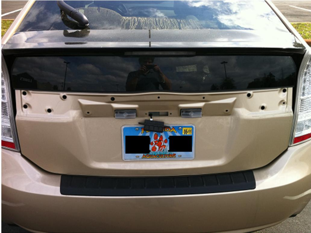
Disconnect the existing hatch release switch and set it aside. I found it easiest to slide the new switch onto the bolts on the trim piece (make sure you don't put it on upside down), then reinstall the trim piece, then connect the wire to the switch from the inside. Finally, put all four bolts back on and reattach the trim panel.
