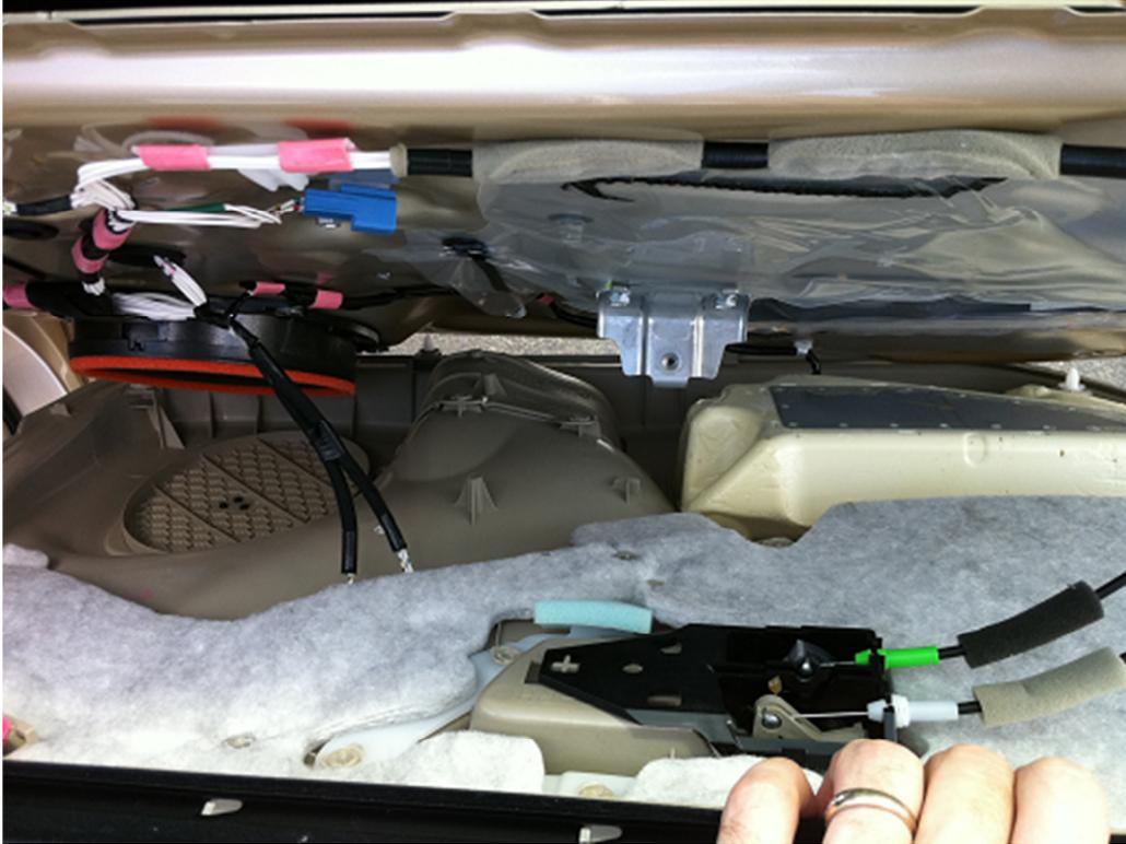
To disconnect the wires just pinch the release and slide the connector out of the socket. They should come out very easily, so if you can't get them out then you probably don't have it released correctly. To disconnect the cables for the door handle and locks, simply pull the cables forward as shown below and pull the ball out of the socket.
