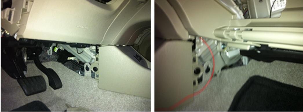
Finally, connect the end of this wire to the lead that you had left disconnect earlier with the diode you got from radio shack between them. The cathode end of the diode (the end with the band) should be connected to the wire that goes to the ECU on the driver's side.
