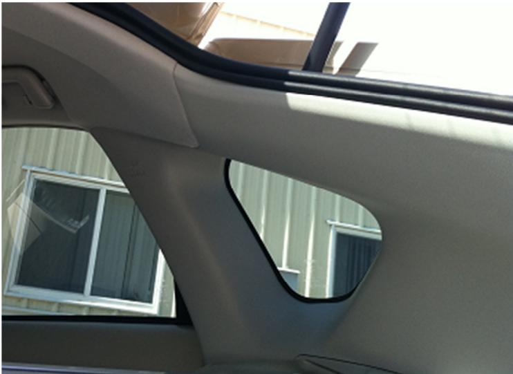
...just by pulling back on it so I could route the wire behind it and bring it out by the rear passenger door. Be careful because there is an airbag behind the headliner above the rear door... you don't want to accidentally puncture the airbag or route the wire over it such that it would get in the way if the airbag deployed.
