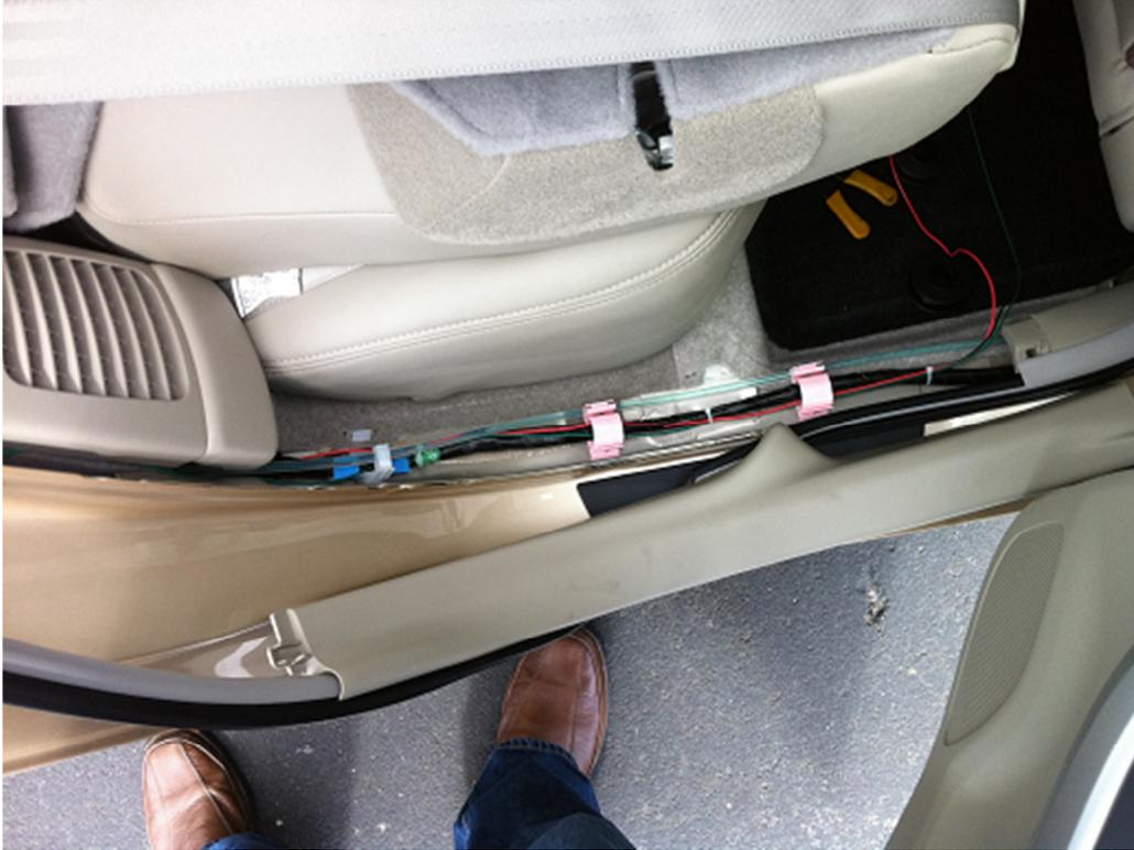
Now open the front passenger door and pull up that door sill... again, it just lifts straight up. I pulled the bottom of the trim on the pillar between the doors out enough that I could run the wires under it without taking it all the way off. Continue running the wires up toward the front of the car.
