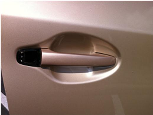
Finally, pull the handle back and out to remove it from the car.
