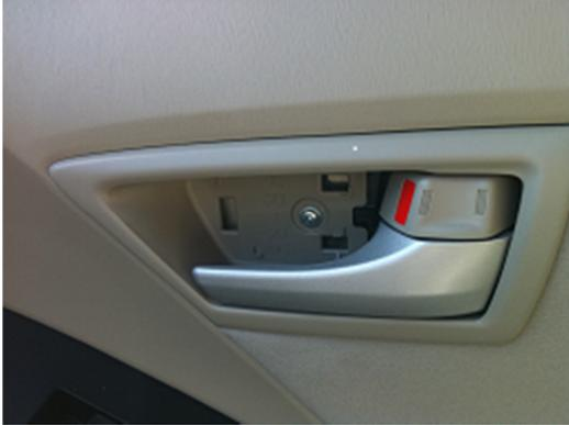
Next lift the rubber piece out of the finger hold on the door. This isn't attached to anything and can just be lifted up.
