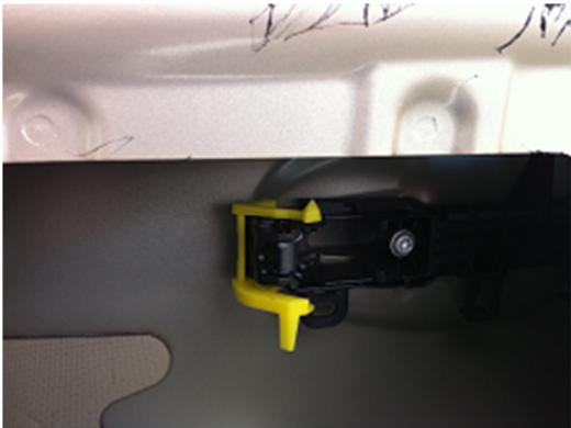
Locate this circular black plug on the side of the door just above the latch.
