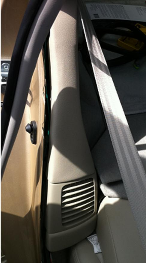
Once you've got the wire routed that far you can, go back and push the trim piece back into place and reattach the headliner (be careful not to pinch the wire against a clip or anything).
