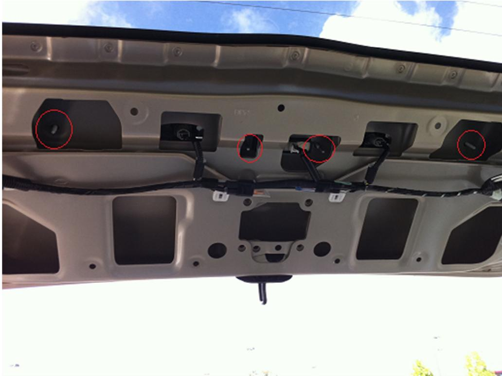
Remove the outside trim from above the license plate. Those four nuts are what hold it on, so once they're removed you can simply pry it away from the car. The hatch release switch is simply slid onto two of the bolts that stay attached to the trim piece, so once that's been removed the switch is no longer attached to anything. You can see the hatch release switch dangling from the cable in the picture below.
