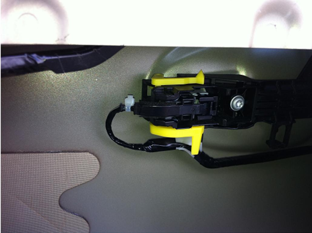
Connect the other end of the new harness to the blue connector that's already on the door and push the white and black locks into the door to hold the harness in place.
