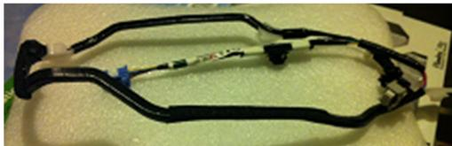
Wiring harness for passenger door SKS handle. \$37.55. Part number 89746-47040. Note that this is for the right hand side. If you have a RHD car or you're trying to enable SKS for the rear doors then you want part number 89746-47050 for the left hand side.
