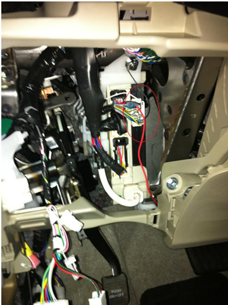
Route that new wire over to the passenger side of the car. I did this by pulling off the trim pieces on the right side of the driver's footwell and the left side of the passenger's footwell, then passing the wire through as the pictures below show.
