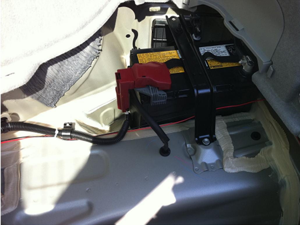
Finally, I tucked them down between the HV battery cover and the side of the car leaving the wires coming out next to the rear seat for now.
