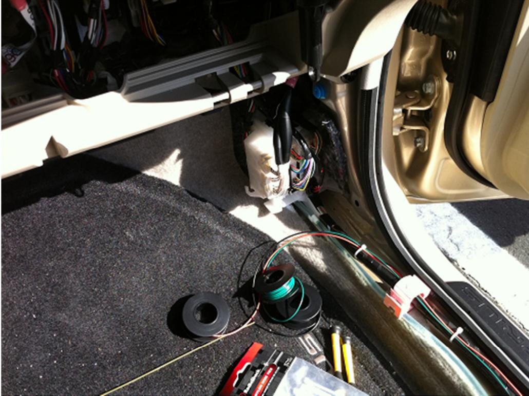
The group of white wires is the harness coming from the passenger door that contains the wires going to the SKS handle we installed earlier. We need to locate the wires that we need from that group. The wires you need to locate are:
