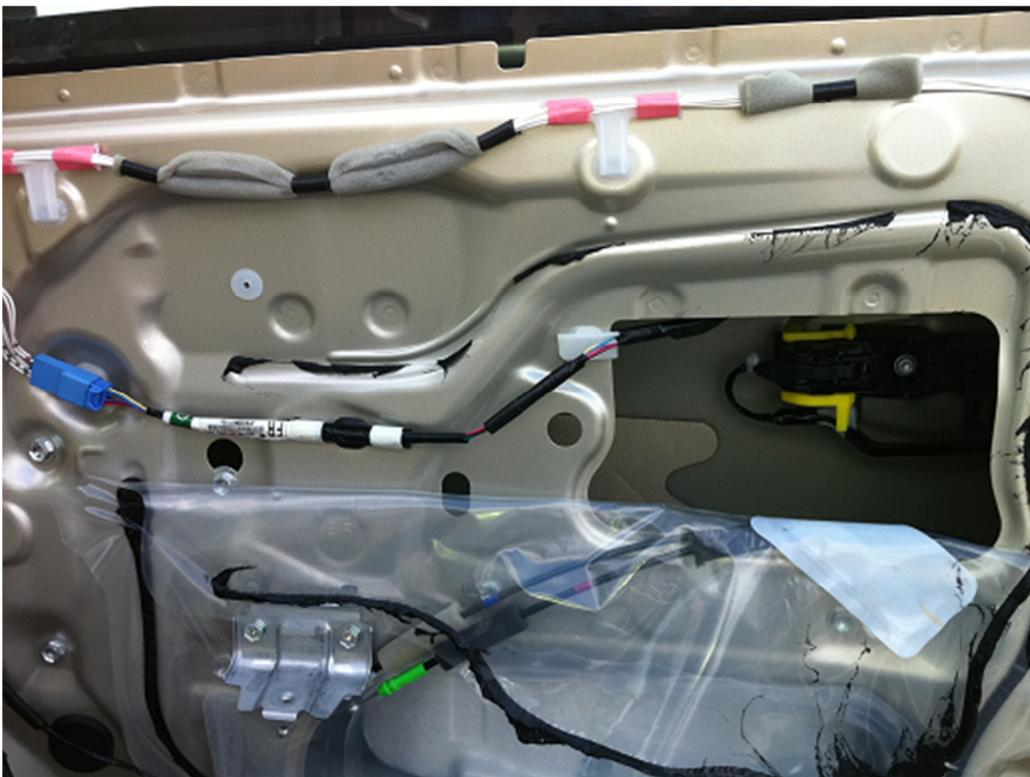
Push the moisture seal back up and run your finger around the edge to reseal it
