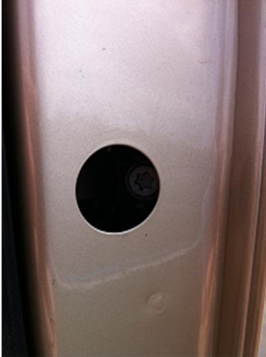
Using a T27 Torx screwdriver loosen the screw. Note that it's a captive screw so even when it's totally unscrewed it won't fall out into the inside of the door. Once the screw has been loosened pull out the small trim piece next to the exterior handle.
