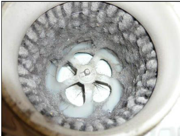
Figure 1. HV Battery Cooling Fan BEFORE Cleaning
