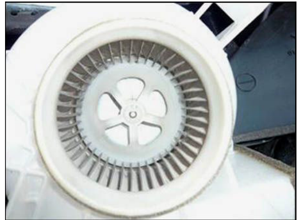
Figure 2. HV Battery Cooling Fan AFTER Cleaning
