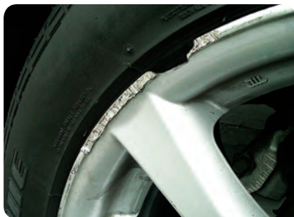
Damaged Alloy Wheel
