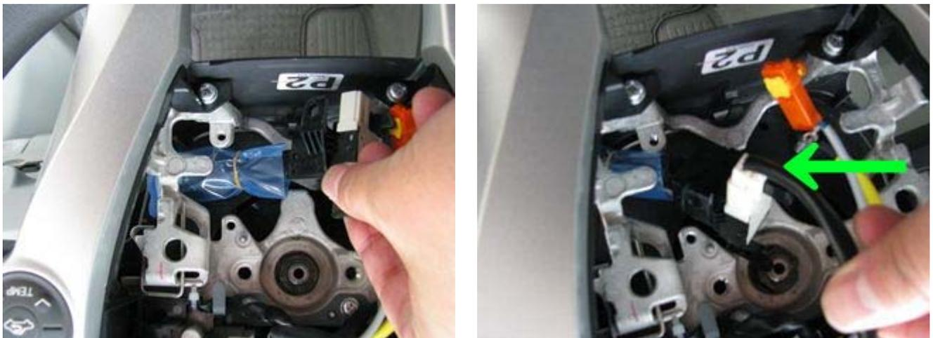
Fasten the cruise control stalk with the two M5x10mm screws (A and B in the picture below). (Alternatively, M5x8, or M5x15 screws can be used).
