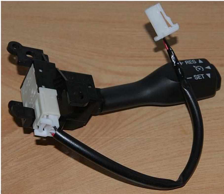
For each switch position, test the resistive values of the switch with an ohmmeter (or multimeter), following the resistive figures previously shown and verify that the purchased unit produces compatible values.
