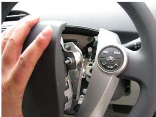
It is suggested to rotate the steering wheel before removing the front block including the airbag.
