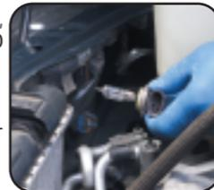
**NOTE:** Only use a bulb with the same part number and wattage rating. Aiming is not necessary after replacing the bulb. When aiming adjustment is necessary, contact your Toyota dealer. Do not get dirt, grease or fingerprints on the bulb; this can cause the bulb to burst or fail prematurely. Dirt or grease can be removed with rubbing alcohol and a clean cloth or lint-free paper towel. The bulb must be dry before installation.
