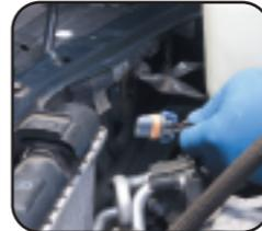
3 TURN THE BULB RETAINING RING COUNTERCLOCKWISE AND REMOVE THE BULB AND RING. On vehicles where the bulb is installed into the connector, simply remove the bulb.
