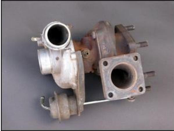
Of the choice between a supercharger and turbocharger, a turbo gives the highest efficiency. This is because it uses heat that's otherwise wasted out of the tailpipe, whereas a supercharger is drawing power directly from the crankshaft. So in terms of fuel economy, a turbo is a better choice.
