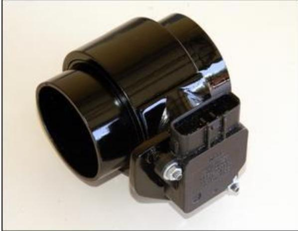
The new airflow meter housing was made from a variety of PVC plastic plumbing adaptors, all available from the local hardware store. These were cut, filed, sanded and heated into shape, with the resulting airflow meter having a minimum internal cross-sectional area 31 per cent larger than standard. The airflow meter was located behind the right-hand headlight. The Digital Fuel Adjuster was then used to boost the airflow meter output signal so that the car ran as normal.
