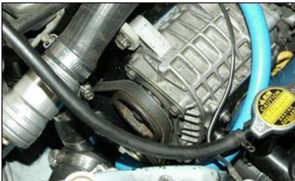
The belt drive had settled down (I gave it greater tension that stopped its whipping) and on the road the car was performing fine. The mixtures were a little leaner than preferable, but that could be easily changed with the Digital Fuel Adjuster.
