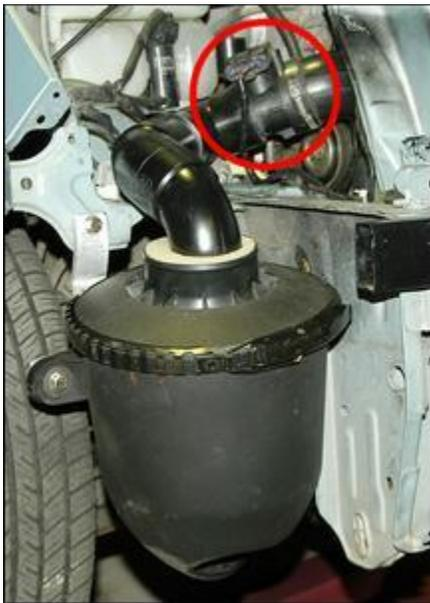
Up until now I'd been using the factory airflow meter, cut from the airbox into which it is normally integrated and mounted in-line after the new Falcon V8 airbox. However, its small size and the slightly bodgie way in which the chopped-up airflow meter fitted into the intake plumbing caused me to reconsider the approach. I decided to kill two birds with one stone and build a new, larger airflow meter that had proper in-line plumbing connections.
