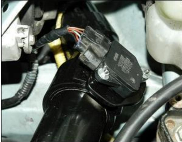
At this stage the airflow meter sensing element was installed in a custom-made body with a 31 per cent larger cross-sectional area. The DFA was then used to lift the output voltage value of the larger airflow meter to achieve correct closed-loop mixtures. New free-flow intake and intercooler plumbing was also installed at this time.
