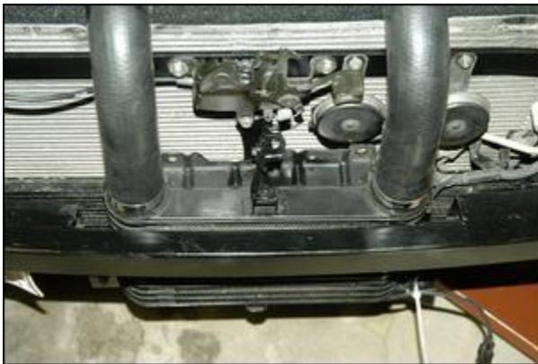
In order that the intercooler could be mounted in this position, the power converter radiator needed to be moved backwards and the frontal intrusion bar modified to provide clearance. I cut out a section of the original bar and then had welded across the gap a section of the bar from the half-cut Prius that I had bought. Note that this bar is slightly curved in plan, so it couldn't just be replaced with straight rectangular tube.
