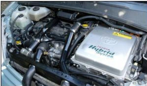
Part of the difficulty in describing the performance change is because the Prius Power Split Device varies engine revs according to speed and throttle position. So to reach peak engine power (as measured by the airflow meter signal), the car needs to be travelling at over 100 km/h at full throttle. At anything less than about 100 km/h, full throttle makes use of the typically much improved mid-range power. (It's improved because there's always plenty of electric power available.)
