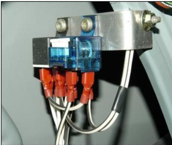
On-road testing showed that the system worked – consistent rich mixtures on high loads with no apparent learning around them occurring. I then added two relays – one the changeover from solenoid-off-to-fuel-pump-on, and the other a power feed relay for both the solenoid and the pump. A second relay was also added to the Simple Voltage Switch to trigger the fuel pressure changeover, so that the oxy sensor switching and fuel pressure switching occurred simultaneously.
