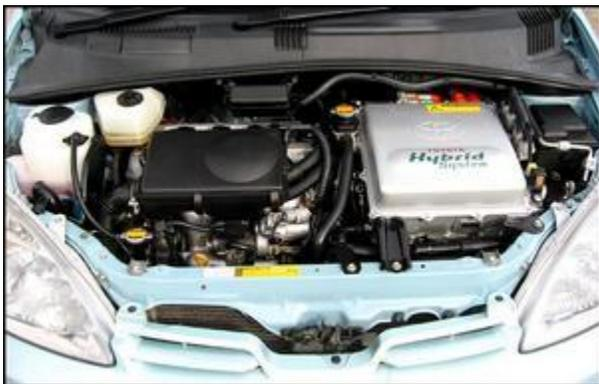
Most important of these differences is that the Prius engine uses what is called an Atkinson cycle. In this approach to valve timing, the inlet valve stays open for a long time – in fact, even as the piston is well into the compression stroke. This forces some of the intake mixture back out into the intake
