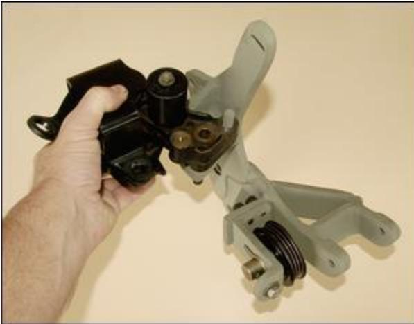
This was primarily because of the very cramped engine bay in the Prius, which necessitated (for example) integrating the supercharger mount into a completely new fabricated engine mount. This bracket was made from mild steel, using 9mm plate, 12mm plate and 40 x 8mm bar, arc welded together. In addition to the heavily gusseted engine mount, the bracket also incorporated the fabricated belt tensioner. In all, something like 40 hours of work went into making the bracket.
