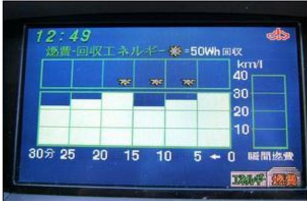
On an open road cruise at 100 km/h, the turbo Prius will turn in a best economy of about 4.6 litres/100km [21.7 km/litre, 61.4 miles per imperial gallon, 51.1 miles per US gallon]. In the same conditions, the dead standard car used to get about 6.3 litres/100 km [17 km/litre, 5.9 litres/100km, 48 miles per imperial gallon, 40 miles per US gallon], so the modified car has improved the fuel economy in these conditions by up to 28 per cent!
