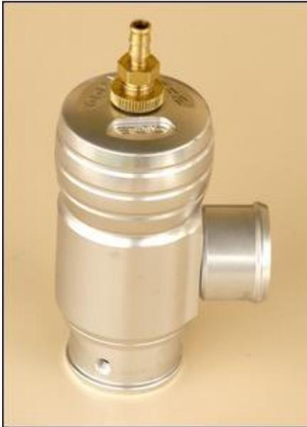
A supercharger bypass valve was incorporated in the system. This comprises a GFB recirculating blow-off valve, normally used on a turbo car. It has 32mm plumbing and is beautifully made. The connections to this valve were plumbed-in just after the airflow meter and just before the throttle body.
