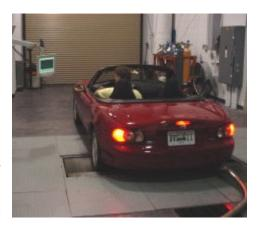
To further exacerbate the issue of inaccuracy with "real world driving", the EPA tests all the cars in a temperature- and climate-controlled building at 68-86 degrees Fahrenheit. For the highway portion of the test, they warm the engine before initiating the test. For the city portion, they cold-start the engine. During both tests, they turn the car's air conditioning off and hills are not simulated. To determine gas usage, the Carbon-Dioxide content of the car's exhaust is measured.
